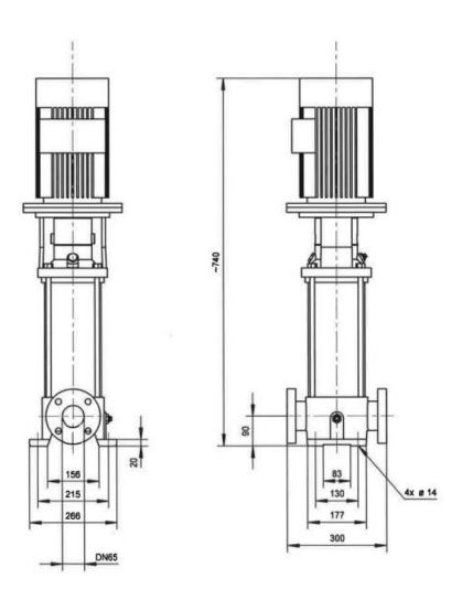
MULG-V 1505 IILG-4.0/2 Centrifugal pump, multistage, vertical, normal priming; with electric motor
